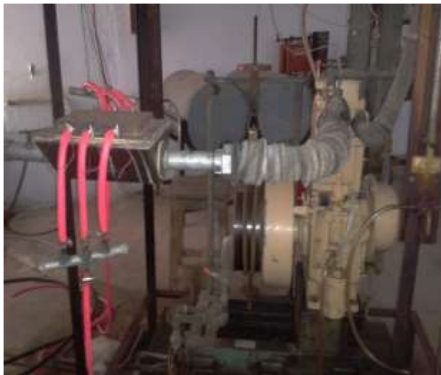
Fig. 3 Assembly of TEG to a CI engine. plate
